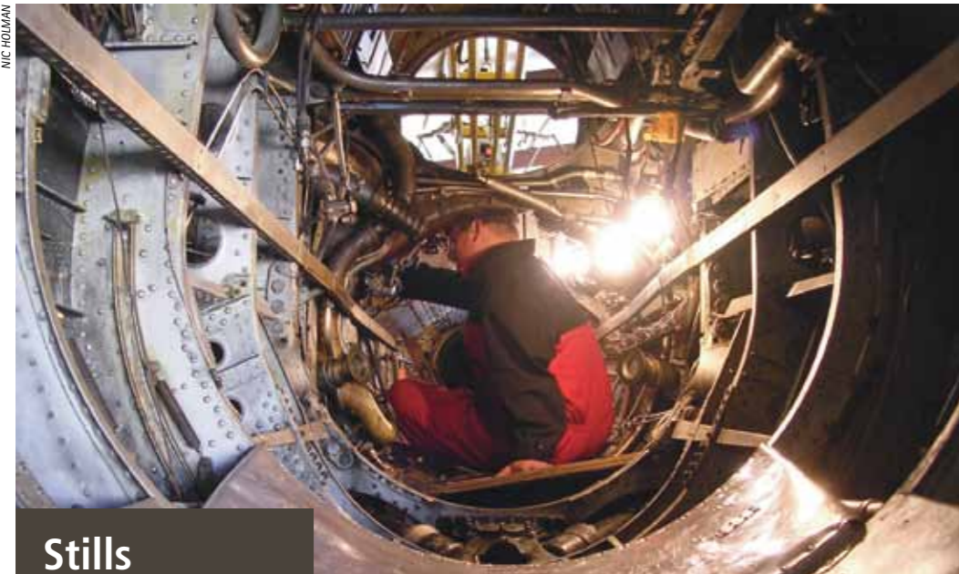
▲ Restoration engineer Dave Tylee working around the air turbine gearbox in the rear fuselage
